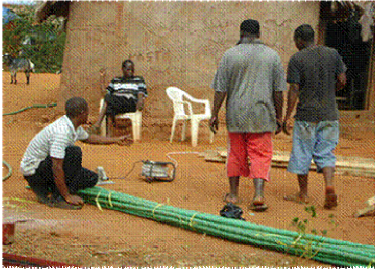
Figure 3. PVC materials ready for cutting to size and melting for fabrication of cages
