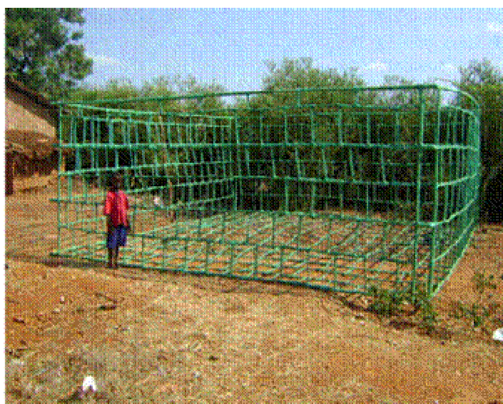
Figure 6. A complete cage 5x5x2m ready for fitting of netting material and landing
