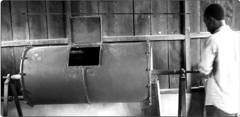
Figure 4.3-2. A hand-operated mixer is used to mix feed ingredients at Sagana Aquaculture Centre.
