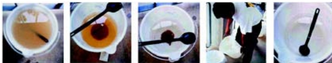
Picture D.1. The PuR process in five steps (P&G, 2004)
