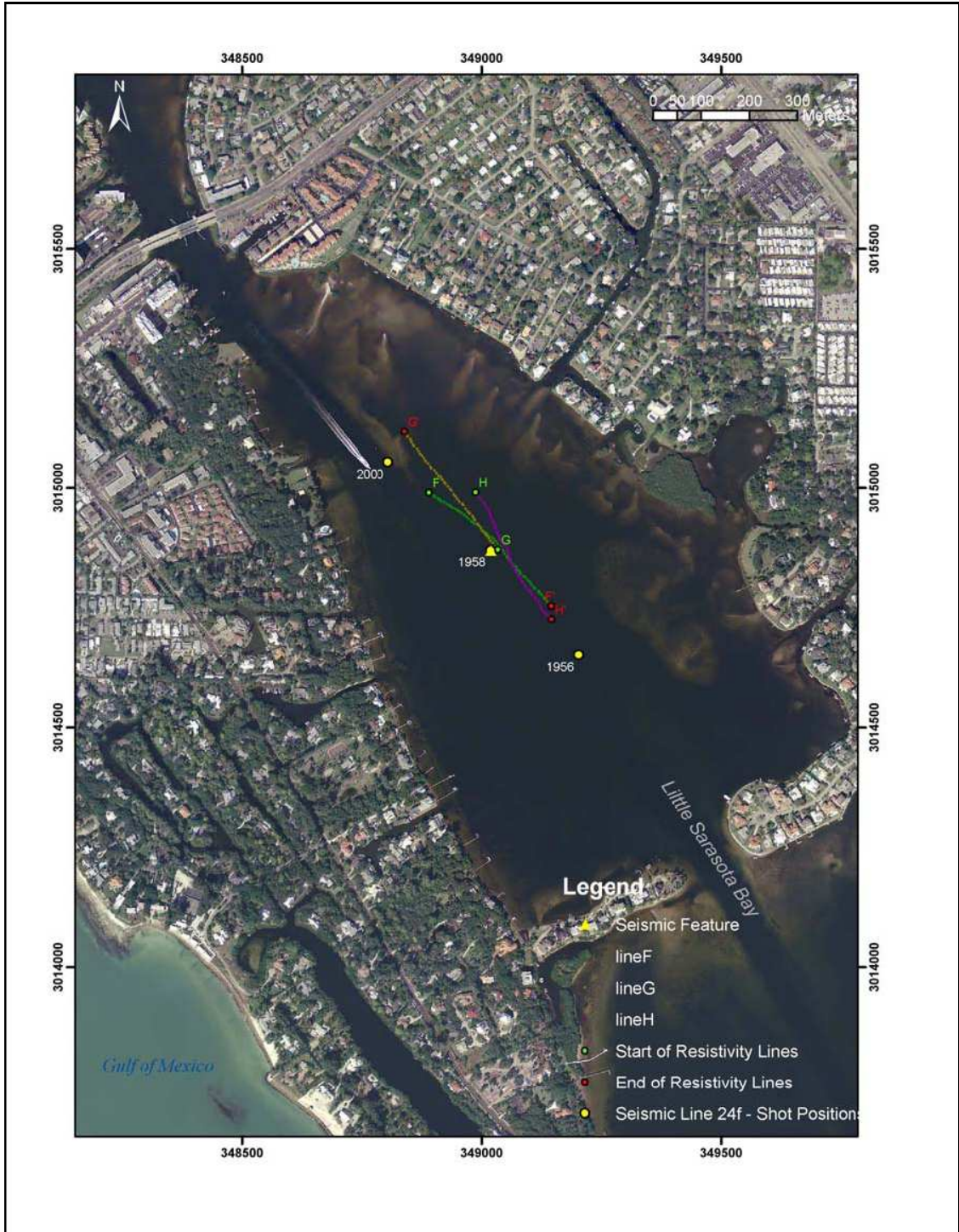
Fig. 4.12b: Locations of resistivity lines F, G, and H run at location of seismic line within the Sarasota Bay system (May'03).
