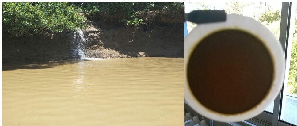
Figure 2. photos of the point of pollution where raw sewage is released into Mtwapa Creek (left) and filtered concentrated Total Suspended Solids (TSS) from water samples collected from the same sampling site (right)
