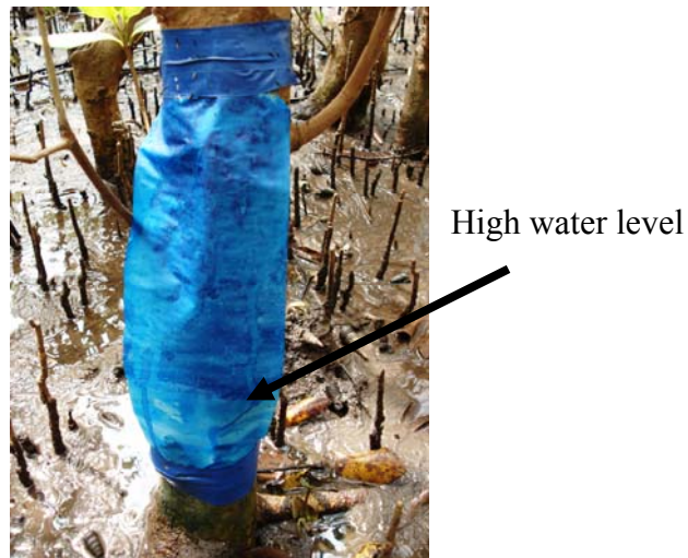
Figure 5. Tracing paper wrapped round a tree showing the level attained by water during the previous high tide.
