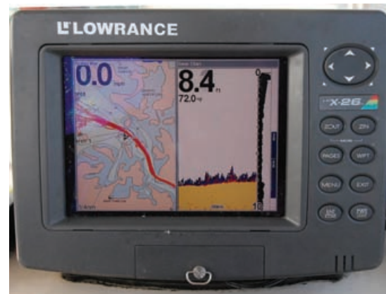
This image of a combination GPS-sonar unit, taken on Lake Marion, South Carolina, shows shallow bottom terrain and surface temperature on the right, and a hydrographic chart and navigational view of the immediate area on the left.
