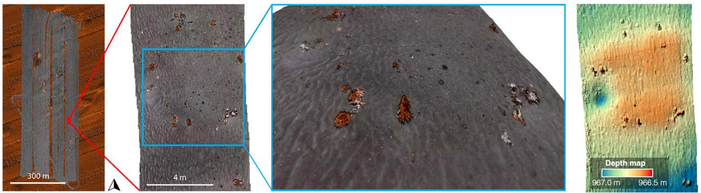
FIGURE 3. Three-dimensional visual mapping data gathered at the Darwin Mounds marine protected area (59°54'N, 7°39'W). The top left panel shows a 30 ha area mapped using BioCam mounted on the autonomous underwater vehicle overlaid on side-scan sonar data. The expanded detail (indicated by red lines) shows a micro-mound (~5 m diameter, 20 cm high). The smaller, individual protrusions that form a ring around the mound are cold-water-coral colonies consisting mainly of Desmophyllum pertusum and Madrepora oculata . These can be seen more clearly in the expanded isometric view indicated by blue lines. The individual colonies have diameters of between 20 cm and 50 cm and are between 10 cm and 30 cm high in the area shown.
