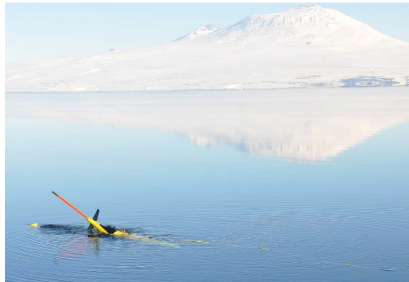
FIGURE 3. A Kongsberg glider is shown deployed in McMurdo Sound, southern Ross Sea. Gliders can be deployed from fast ice around Ross Island, transit to their study sites, and then be recovered from vessels. Photo credit: Vernon Asper
