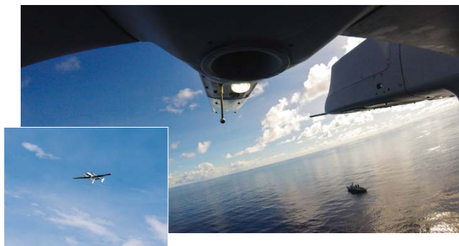
FIGURE 3. During the 2019 R/V Falkor expedition, the team tested the new capabilities of high-endurance hybrid fixed wing vertical take-off and landing (VTOL) UAV (inset) for oceanographic applications. Pictured is the underside of one of the aircraft, making a pass of the ship. Photo credit: Alex Ingle/Schmidt Ocean Institute
