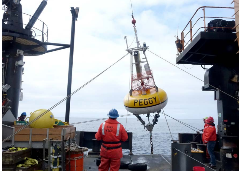
FIGURE 2. Deploying the M2 “Peggy” mooring from NOAA Ship Oscar Dyson on an unusually calm spring day in the Bering Sea. The surface mooring was named after Peggy Dyson, who for many years (1965–2000) broadcast the marine weather on WBH-29 Kodiak for more than a dozen meteorological areas along Alaska’s coast. She was the voice of the north and wife to fisherman Oscar Dyson, namesake of the NOAA vessel in this photo.
