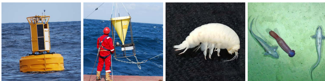
FIGURE 1. The Porcupine Abyssal Plain Sustained Observatory monitors essential ocean variables from the atmosphere to the seafloor (4,850 m), with a satellite-linked surface buoy, sediment traps deep in the water column (3,000 m), the collection of specimens including scavenging crustaceans near the seafloor, and photographic surveys of wildlife nearly 5 km beneath the sea surface.
