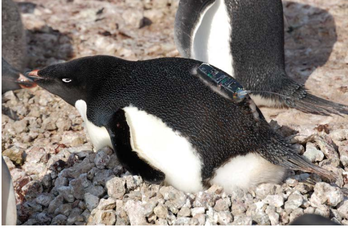
FIGURE 2. An Adélie penguin with an attached bio-logger. The sensors are attached using Tesa tape and are easily removed when penguins return to land. Previous investigations have shown that such bio-loggers do not impede penguin foraging or survival. Photo credit: Jean Pennycook
