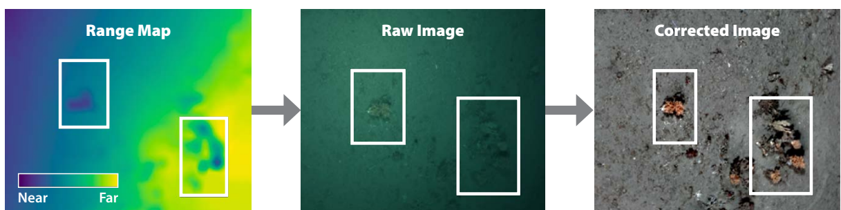
FIGURE 2. Laser-derived 3D range information is used to rectify the color information in the images. Physics-based image formation models use the range maps to compensate for the wavelength-dependent attenuation of light in water. This allows the darkening effects and the blue-green hue seen in the raw images to be rectified even over rugged terrains.
