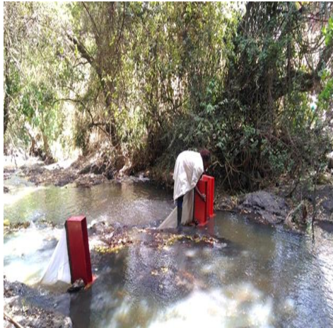
Plate 1: The riffle biotope in the Njoro River showing the researcher positioning a drift sampler at the right bank facing upstream Source: Author
