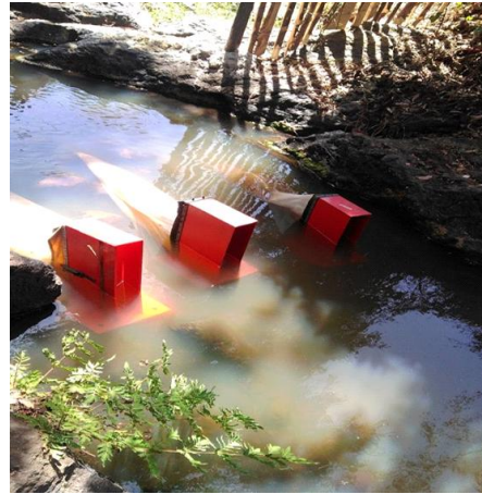
Plate: The pool biotope in the Njoro River showing the drift samplers at different positions Source: Author
