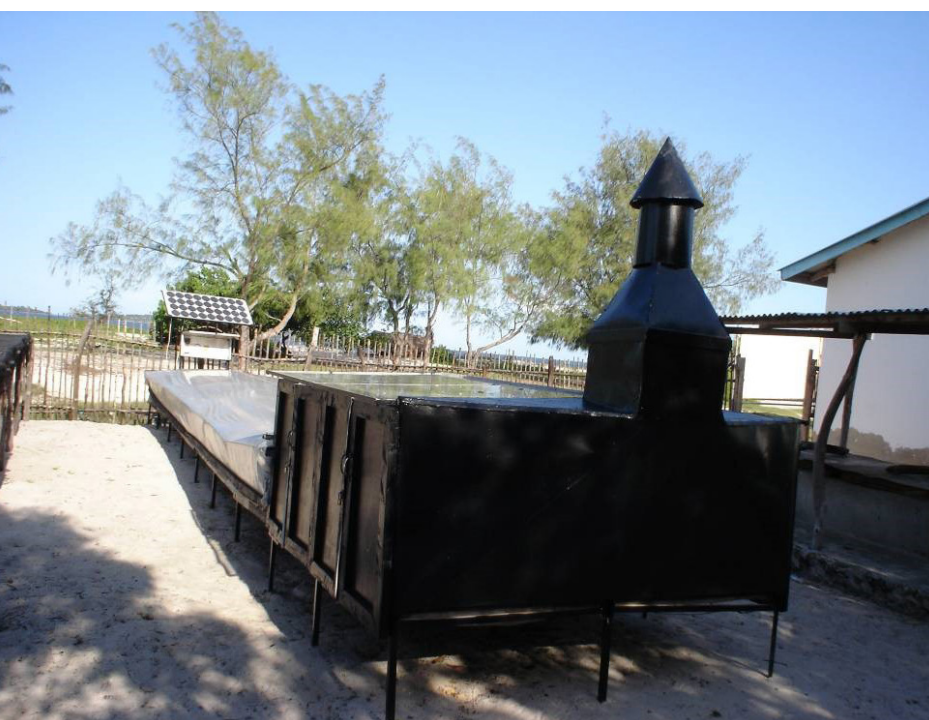
Fig. 1: Solar tunnel fish dryer
