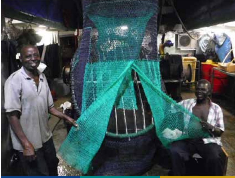
Mr Rashid Anam (KMFRI and vessel crew) with the new TED mounted on the trawl net. © Michel Nalovic
