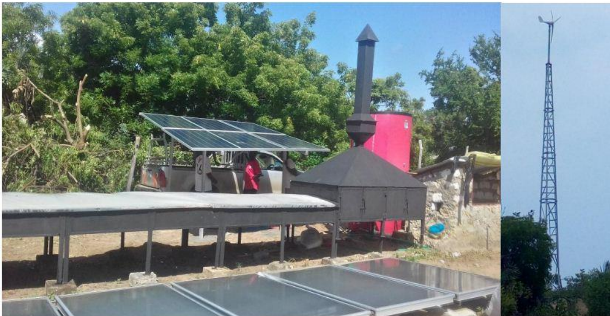
Figure 2.9: The drying system of the hybrid windmill solar tunnel dryer in Kipini showing the tunnel dryer, drying chamber, windmill and hot water system
