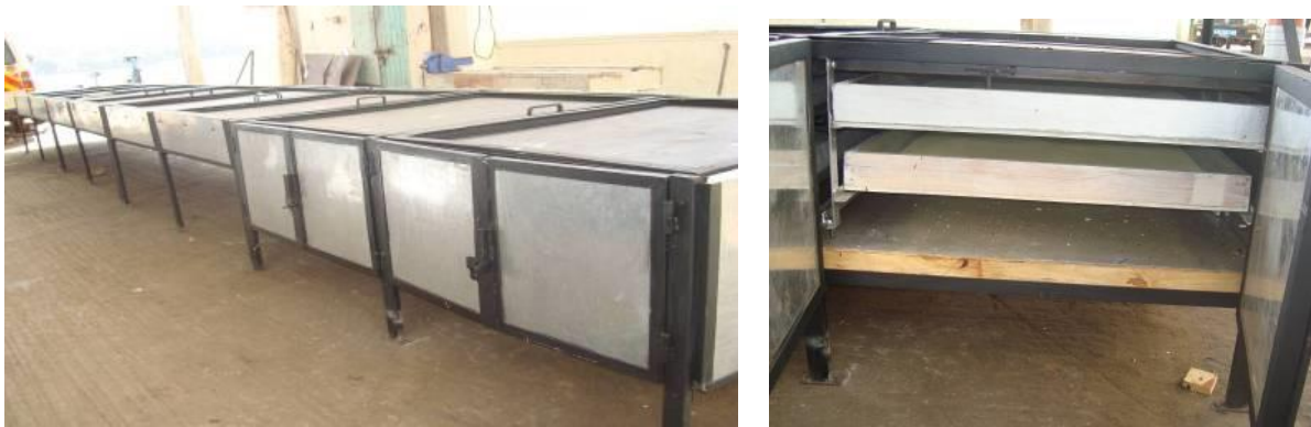
Figure 2.2: a) The collector and hot air chamber
