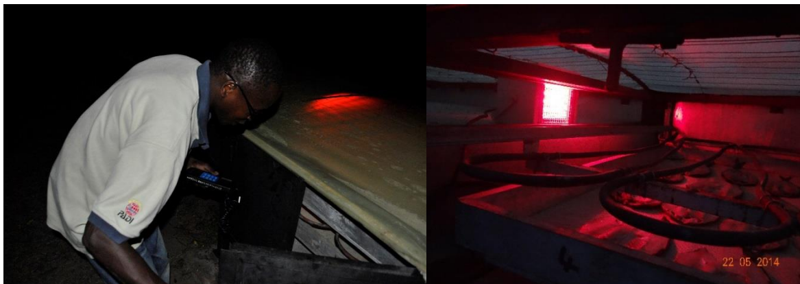
Figure 2.6: DC coil glowing with heat in drying chamber of the hybrid windmill solar tunnel dryer in Kipini, Kenya
